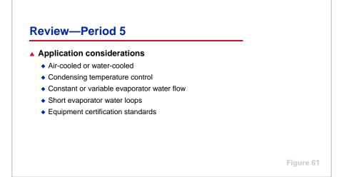
In Period 5, several considerations in the application of helical-rotary water chillers were presented. These included air-cooled or water-cooled condensing, condensing temperature control, constant or variable evaporator water flow, short evaporator water loops, and equipment certification standards.
